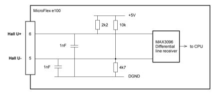
Figure 13 - Hall channel input circuit - U phase shown
